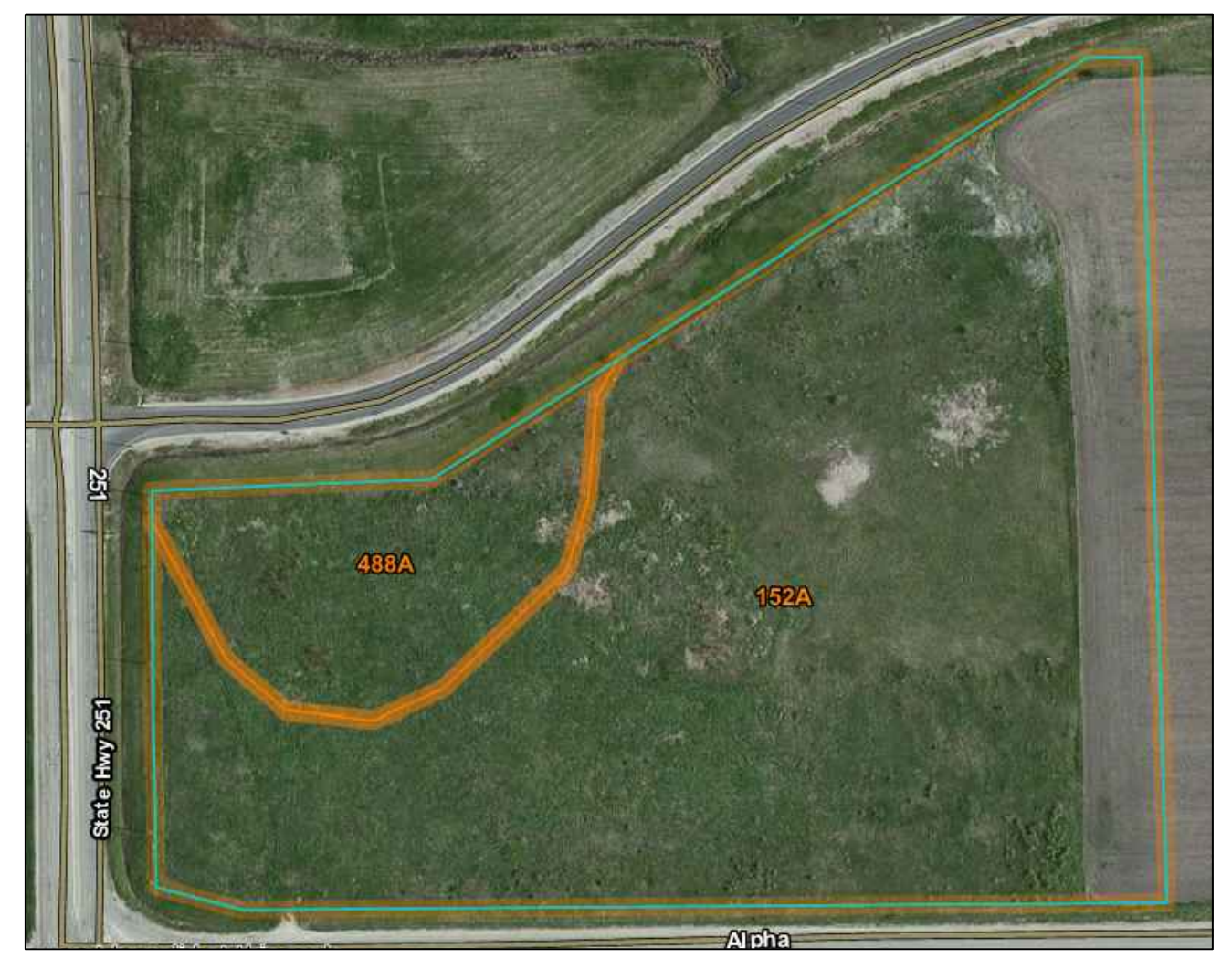
(TYPE B/D) - 152A - DRUMMER SILTY CLAY LOAM, 0-2% SLOPES (85.8%) (TYPE B/D) - 488A - HOOPPOLE, 0-2% SLOPES (14.2%)
