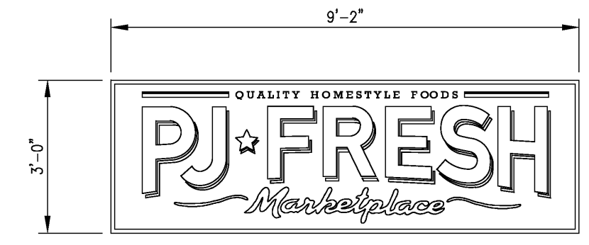
09 SQUARE FOOTAGE: 27.50 SF. PJ FRESH IMAGE LETTERS: WHITE AND GREEN (PMS# 366) BACKGROUND: BLACK INTERNALLY ILLUMINATED, SINGLE FACE WALL SIGN WITH BLACK CABINET AND RETAINER.
